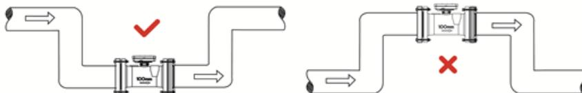
When installed at a U-bend, the meter should be positioned at the lowest point. Air can accumulate at higher points in the pipe, leading to inaccurate or failed measurements.
